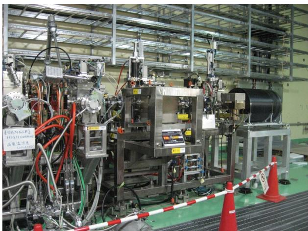
Figure 5: MEBT, D-Plate and LPBD.
