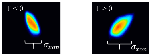
Figure 2: Electron beam profiles. Measured beam sizes varied when the polarity of deflection changed.
