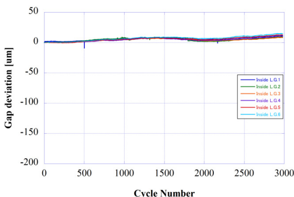
Figure 5: Result of load cycle test with additional nuts.
