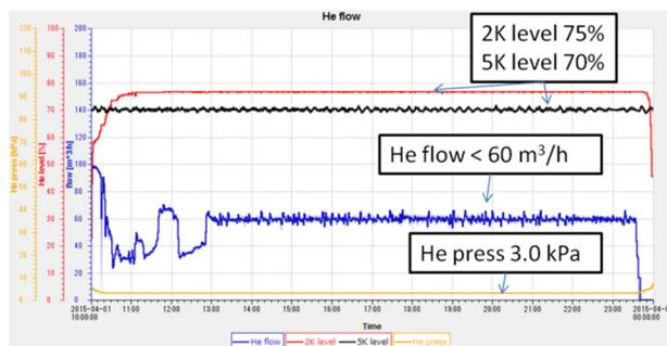
Figure 8: He-gas flow, He-pressure at 2 K, and He level (5 K & 2 K).
