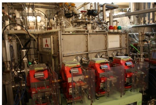
Figure 2: Injector cryomodule at the beam line.
