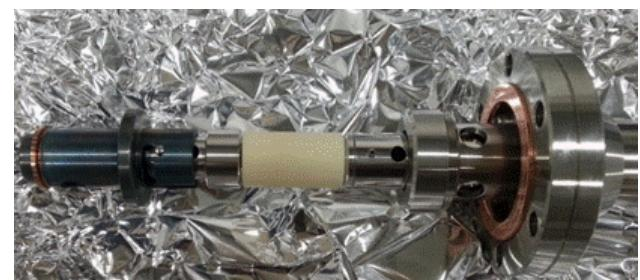
Figure 3: Photograph of the cathode plug and mount of the cathode. The cathode plug is electrically isolated from the vacuum chamber to enable measurement of photo-induced current and quantum efficiency of the cathode.
