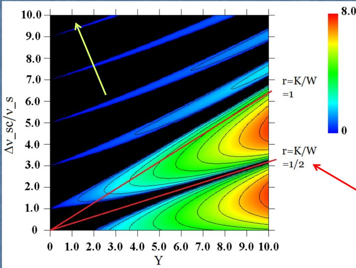
As the space-charge force increases, Eqs. of motion approach to those for two pendulums connected with a spring.
