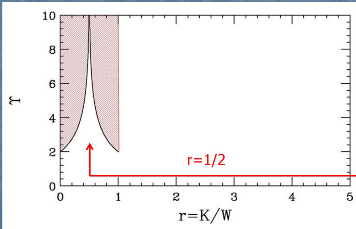
The stability diagram for the weak space-charge case ( $r=K/W \leq 1$ ).
