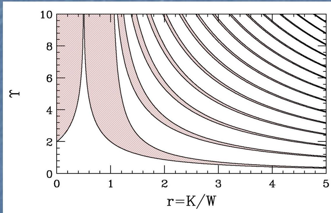
The stability diagram for the strong space-charge case ( $r = K/W \geq 1$ ).
