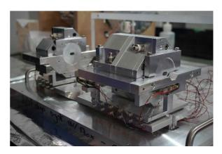
Figure 7: Cavity BPM on piezo mover.
