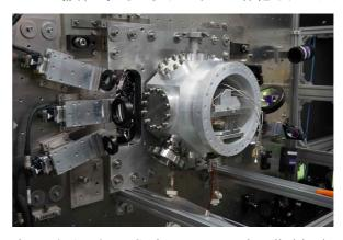
Figure 6: ATF2 IP. Cavity BPM were installed in the vacuum chamber. Closed flanges will be replaced by the viewports for lasers.
