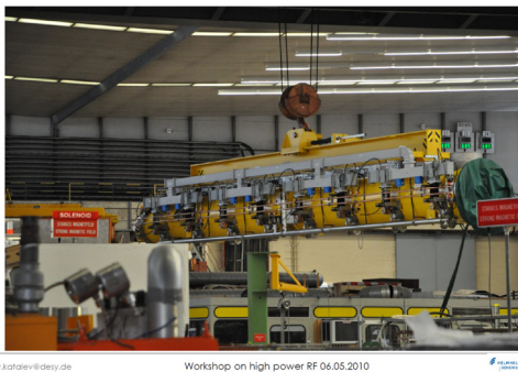
Figure 2: PDS assembled with cryomodule which is used in Euro-XFEL.
