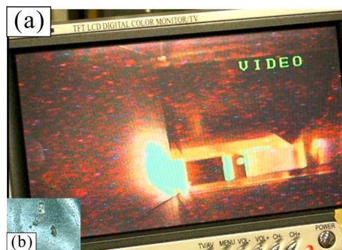
Figure 6: Discharge in the ACS11 circulator. (a) is the arc picture of the discharge and (b) is metallic materials causing the discharge.
