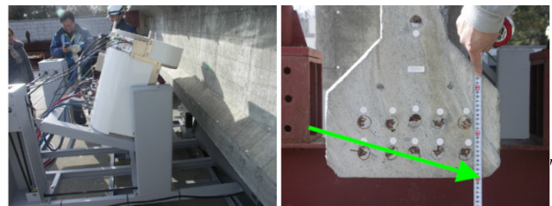
(a) X-ray source and cut sample of real bridge
