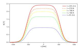
Figure 4: The measured magnetic field along beam trajectries at respective excitation current. The length of BM10 is  $\pm$  550 mm.
