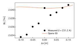
Figure 5: The measured BL products along beam trajectries of dipole field (I = 231.2 A).
