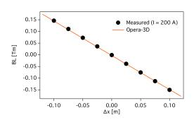
Figure 6: The measured BL products along beam trajectries of quadrupole field (I = 200 A).
