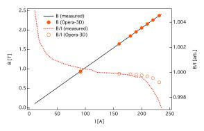
Figure 3: The excitation current dependence of magnetic field (BM10). Light and right axes show B and B/I, respectively. Plotted B/I are normlized by the constant value around I = 120A.
