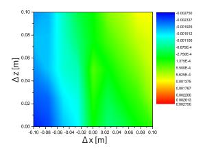
Figure 7: The measured uniformity of BL products along beam trajectries of dipole field (I = 231.2 A).
