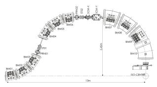
Figure 2: A schematic drawing of the beam-line for the rotating gantry.
