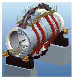
Figure 1: A conceptional drawing of the rotating gantry.
