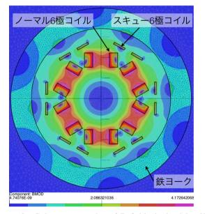
Figure 2: Color contour plot of B-field obtained by 2D magnetic field analysis for HER-SLY magnet. Normal and skew sextupole magnets are excited.
