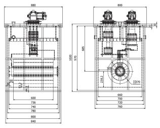
Figure 3: Schematic drawing of the R&D cryostat.
