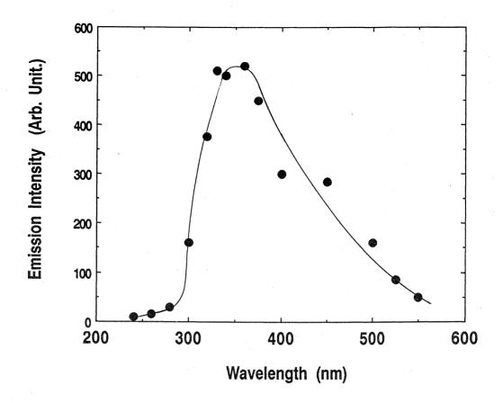
Fig. 2 Emission spectra monitored during 10 ps electron pulse irradiation of Desmarquest AF 995 R at room temperature.
