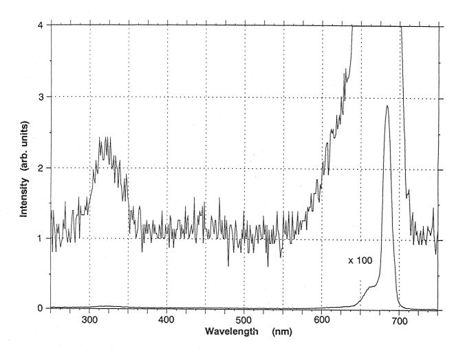
Fig.1 Emission spectra observed by optical multichannel analyzer (OMA) for Desmarquest AF 995 R irradiated with 1.0 MeV H<sup>+</sup> at room temperature in vacuum chamber. H<sup>+</sup> from a single-ended Van de Graaff accelerator.
