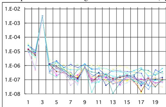
Figure 4: Amplitude of the harmonic components of the magnetic field flux in the long coil. Data were taken and shown for six times each for three sextupole magnets.
