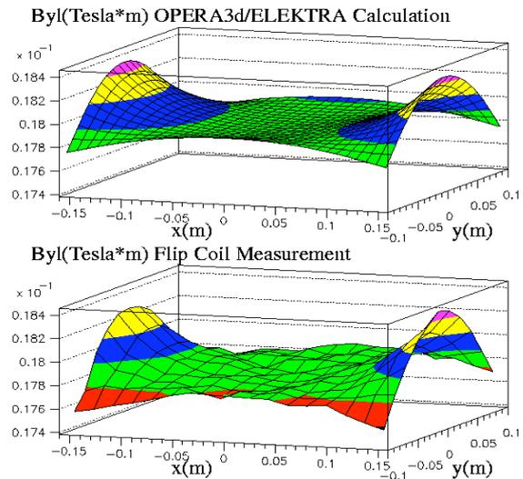
Figure 2: The top figure shows the ELEKTRA calculation of the integral of the y component of the magnetic field with respect to z between  $-0.6$  m and  $0.6$  m,  $B_{yl}$ , by the steering magnet CHN as a function of x and y. The bottom figure shows the flip coil measurement of the field integral  $B_{yl}$ .
