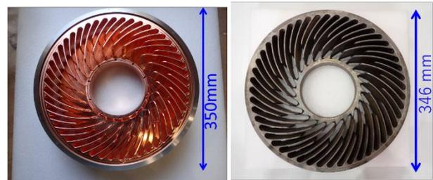
Figure 3: Photographs of prototypes for the rotating-disk-type target. The left photograph shows the Gold-Copper disk model (note: the outside ring is made of heavy metal as a dummy weight). The right photograph shows a trial production made of pure tungsten.
