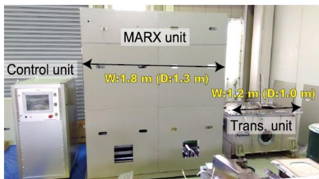
Figure 2: Exterior of modulator. From left, Control unit, MARX unit, Trans. unit.
