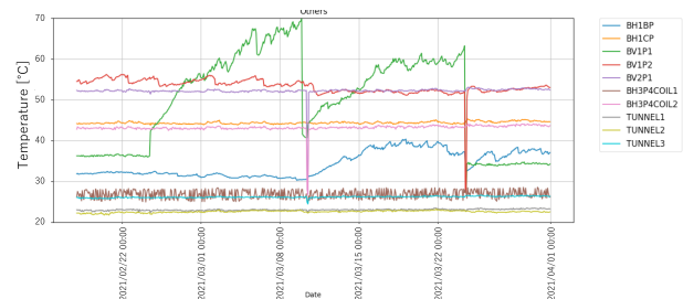
Figure 4: Graph shows the trend of temperatures for BT magnets. The flow rate of cooling water is indirectly monitored using this data.
