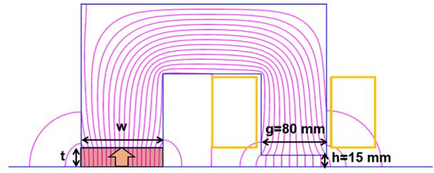
Figure 7: A magnetic circuit of a C-shaped magnet.
