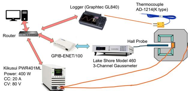
Figure 2: Schematic view of the experiment system.
