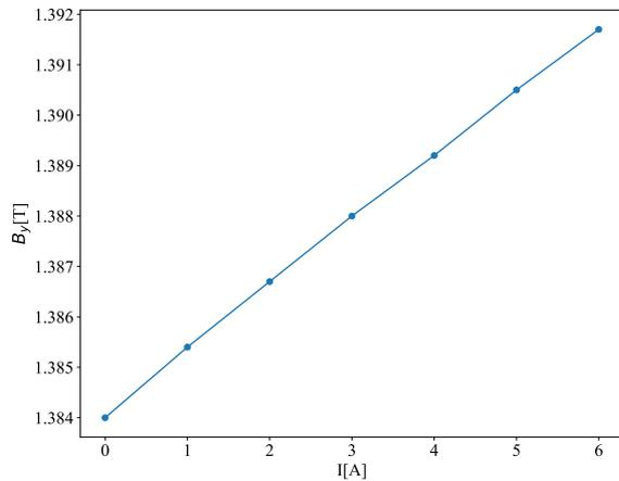
Figure 3: Relationship between magnetic flux density and current.
