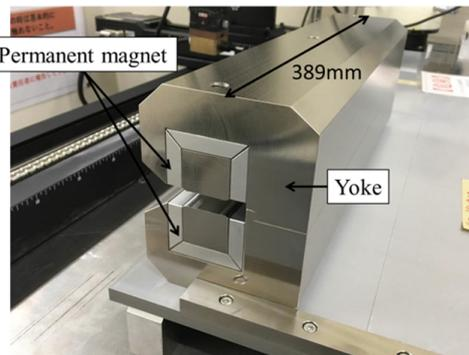
Figure 1: A reduced-scale permanent magnet-based dipole magnet.
