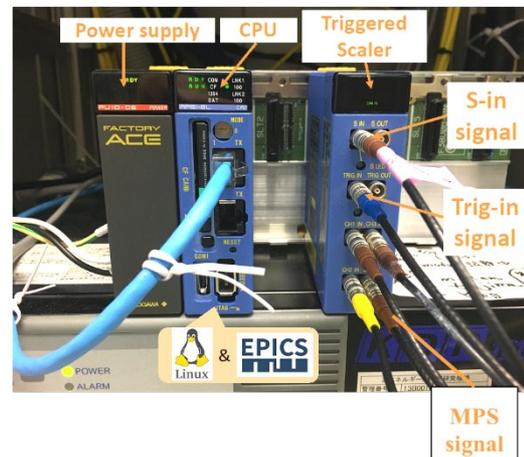
Figure 4: Visualization system of MPS alarms with triggered accelerator scaler module.
