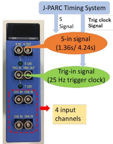
Figure 2: Front view of triggered scaler module.
