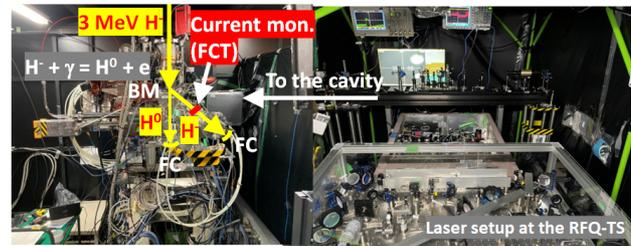
Figure 4: Setup of the laser system for 3 MeV  $\text{H}^-$  beam neutralization study at J-PARC RFQ-TF. The neutralization fraction is obtained by measuring the  $\text{H}^-$  signals with laser ON and OFF by the FCT.
