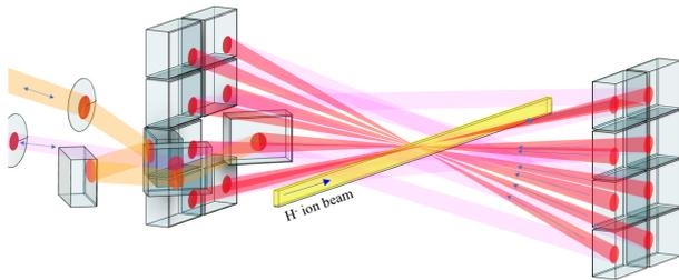
Figure 3: A schematic view of multi-reflection YAG cavity laser system for 32 passes, which was also successfully tested for 3 MeV  $\text{H}^-$  neutralization.
