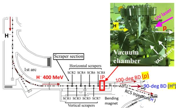
Figure 11: A schematic view of the L-3BT, where a vacuum chamber has been installed for the POP test.
