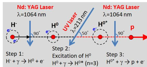
Figure 1: A schematic view of the principle of H<sup>-</sup> stripping to proton by using only lasers at J-PARC. Noted parameters are optimized for 400 H<sup>-</sup> beam energy.
