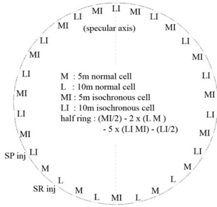
Figure 1: Lattice structure of the PF-HLS ring
