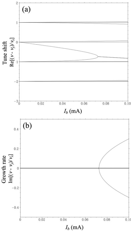
Figure 2: (a) Tune shifts and growth rates of vertical betatron oscillations normalized by synchrotron tune  $\nu_s$  at  $\xi_y = 0$  for  $0 \leq I_b \leq 0.1$  mA. Transverse mode coupling instability occurs at  $I_b = 0.073$  mA.
