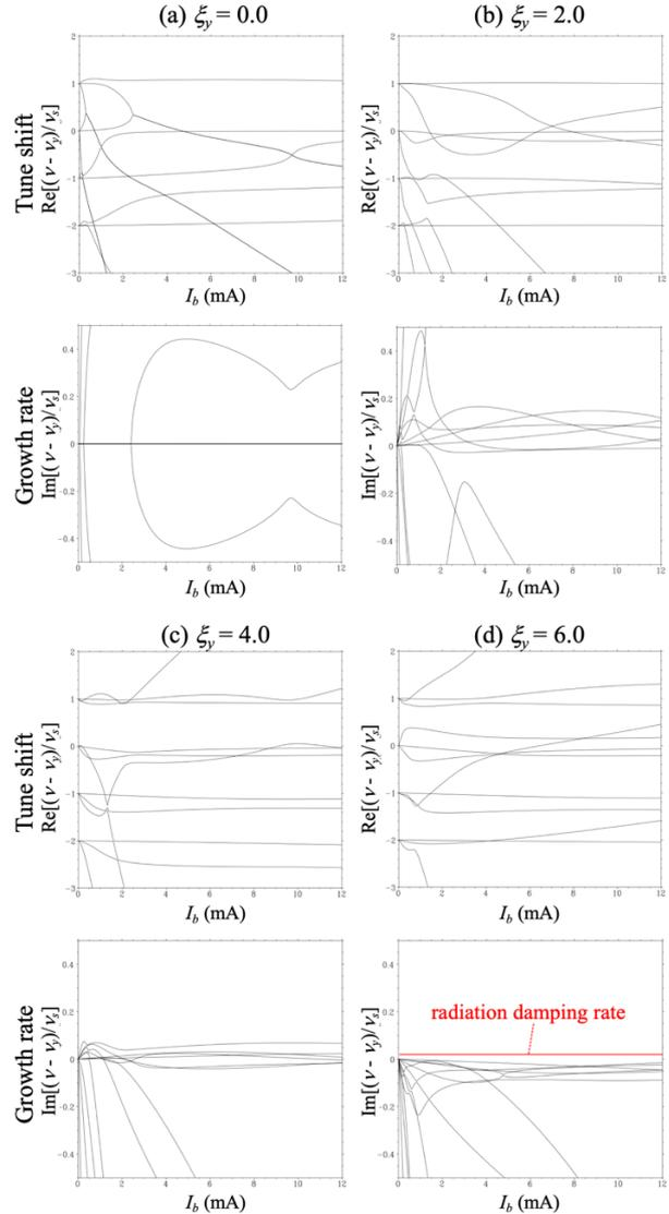
Figure 3: Tune shifts and growth rates of the head-tail oscillations normalized by  $\nu_s$  with (a)  $\xi_y = 0$  (b)  $\xi_y = 2$  (c)  $\xi_y = 4$  and (d)  $\xi_y = 6$  for  $0 \leq I_b \leq 12$  mA.
