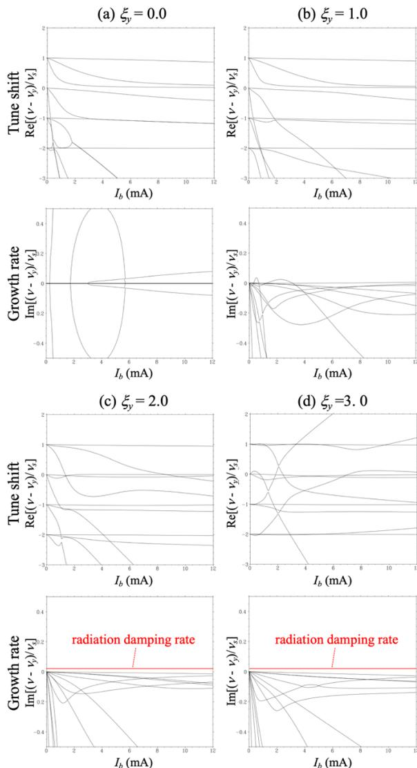
Figure 4: Tune shifts and growth rates of the head-tail oscillations normalized by  $v_s$  with (a)  $\xi_y = 0$ , (b)  $\xi_y = 1$ , (c)  $\xi_y = 2$  and (d)  $\xi_y = 3$  for  $0 \leq I_b \leq 12$  mA.
