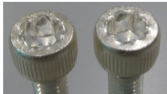
Figure 1: Hex socket head bolt with broken socket hole (strength class A4-70).
