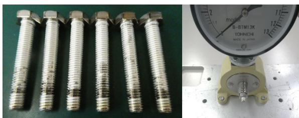
Figure 2: (Left) Discarded Teflon-coated silver-plated bolt (SUS316L), (Right) View of axial force measurement with washers in position.
