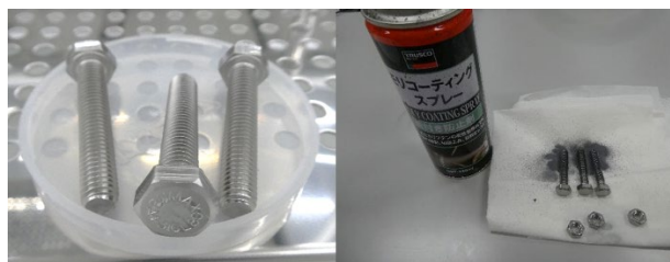
Figure 5: (Left) BUMAX bolts with clean bolt treatment. (Right) Bolts coated with molybdenum disulfide lubricant.
