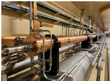
Figure 11: S-band high gradient travelling-wave-type beam-accelerating structures installed in the beam line.
