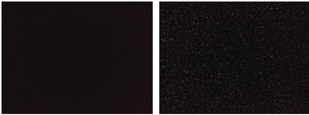
Figure 2: Raw Image Data (ISO : 400, Exposure : 1000 ms @ Downstream of Superconducting wiggler in PF). The image on the left is without beam (NO radiation). The image on the right is with a beam (radiation).
