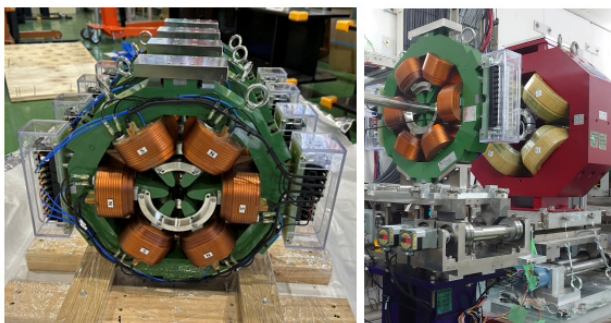
Figure 6: New skew sextupole magnets. These magnets were installed to the ATF2 beamline on May 2024.
