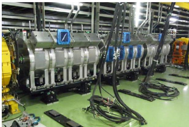
Figure 9: Reassembling work of the RF cavity at MR in 2023 summer.
