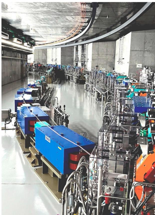
Figure 3: Photograph of 3-GeV beam transport line and injection point of storage ring.
