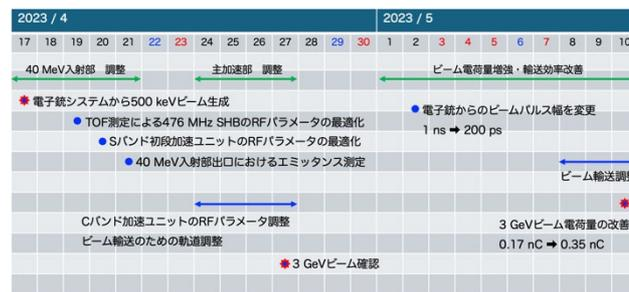
Figure 4: Timeline of beam commissioning 3-GeV linear accelerator.
