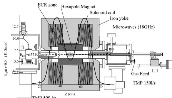
Figure 1: Cross-sectional diagram of the R18GHz ECRIS.
