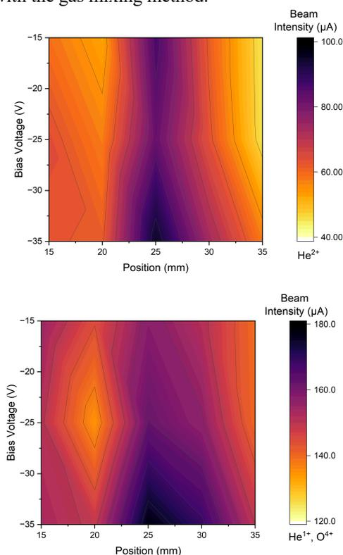
Figure 5: 3D Contour plot of the beam intensity of  $\text{He}^{2+}$ (top) and  $\text{He}^{1+}/\text{O}^{4+}$ (bottom) with respect to the applied bias voltage and disc position along the beam axis at constant microwave power 200 W.
