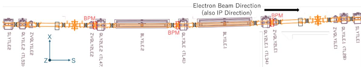
Figure 1. Magnet arrangement between two strong sextupole magnets, SLYTLE1 and SLYTLE2, in the HER (top view).
