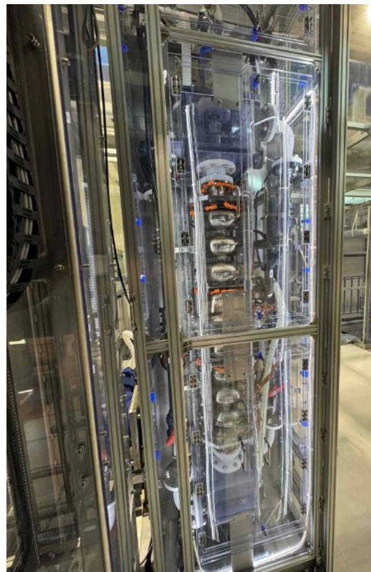
Figure 1: Picture of Nb cavity set in VEP facility at COI building.
