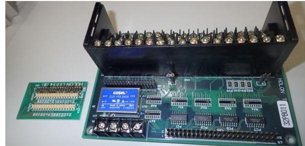
(c) After removing LED board, converter appears.
