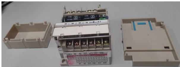
Figure 4: Remove the covers from the frame body. Bottom cover is fixed to the frame body by 6 locking crawls. By using flathead screw driver, you may push all the craw and lever open the cover gradually. All the crawls being disengaged from holes, cover comes off.
