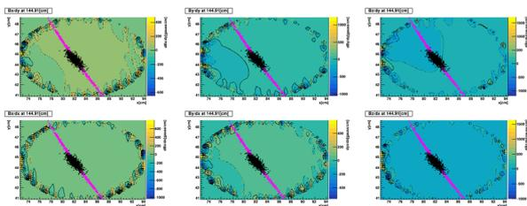
Figure 3: First order partial derivatives of the magnetic field in the channel at  $Z=145\text{cm}$ . The upper row shows the partial differential of the y component of  $B_x$ ,  $B_y$ , and  $B_z$ , and the lower row shows the partial differential of the x component.
