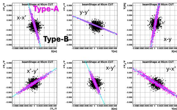
Figure 6: Phase spaces in the beam coordinates at  $z=95\text{cm}$ , point-A as in Fig. 1. Here, the beam coordinate system has the beam center as the origin and the direction of movement as the Z axis. The figure shows the phase space  $X-X'$ ,  $Y-Y'$ ,  $X-Y$  in the horizontal direction (on the X-Y plane) of the beam coordinate system in the upper row, and the lower row shows  $X'-Y'$ ,  $X-Y'$ ,  $Y-X'$ .
