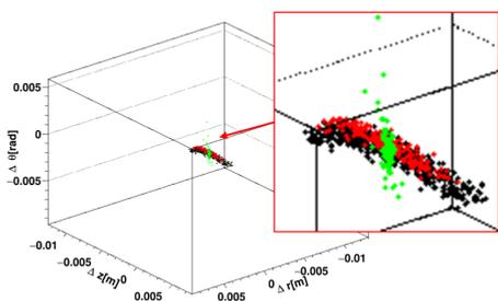
Figure 12: The same data set as in Fig. 11 but expressed differently, in the coordinate system centered on the storage magnet. The radial distance is deviations from the reference orbit  $\Delta r$ ,  $\Delta z$  and the angle between the each particle's position vector and momentum vector  $\Delta\theta$ .
