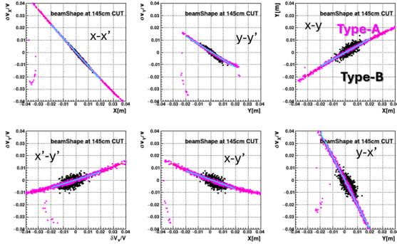
Figure 7: Phase spaces in the beam coordinates at  $z=145\text{cm}$ , at injection point as in Fig. 1.
