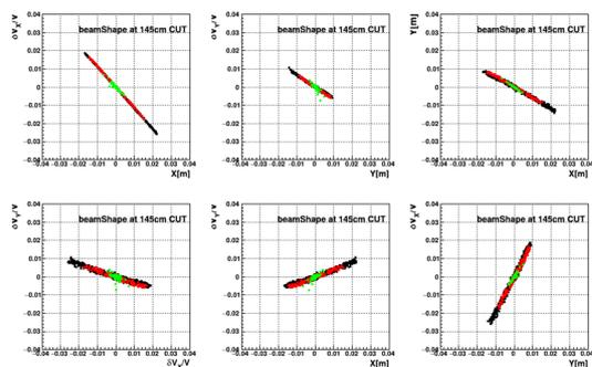
Figure 11: A comparison of four-dimensional phase spaces at  $Z=145\text{cm}$  is shown. Black is ideal for Type-A, the red color is a model that is generated based on singular vectors. Green colored phase space distribution is obtained by the previous methods [2,3], assuming expected emittance from the upstream design.
