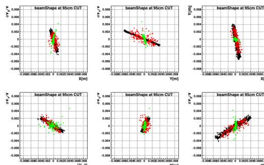
Figure 13: Beam phase space at  $Z=95\text{cm}$  is shown. A difference introduced in Fig. 12 causes the bigger differences among black, red and green distribution at  $z=95\text{cm}$ , although there is no obvious difference in Fig. 11.
