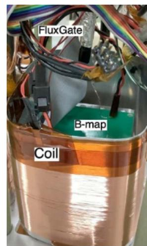
Figure 4: Coil and Flux Gate for calibration.
