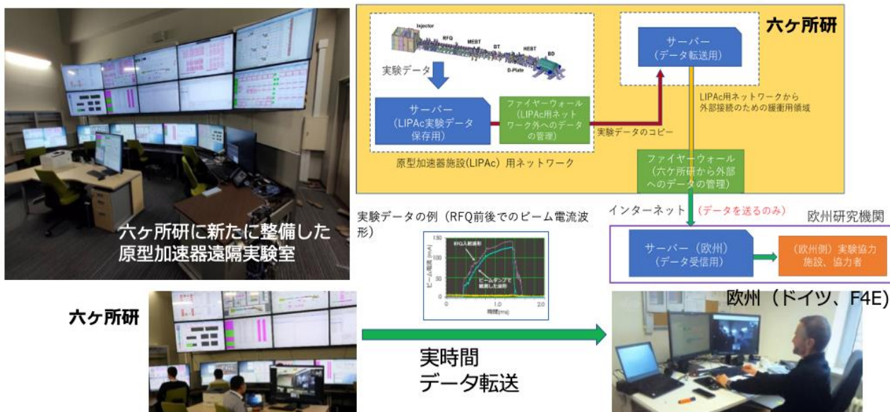
Figure 3: Real time data transfer system from Rokkasho to F4E and schematic view of remote participation from Europe.
