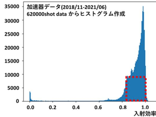
Figure 3: Injection efficiency ( $Q$ -ratio) for the Linac HER beam (electron beam).
