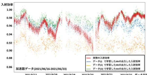
Figure 8: Predicted injection efficiencies (Q-ratios) by DNN with dataset (i) (blue), (ii) (orange), and (iii) (green), and actual injection eff. (red), for 2021 June evaluation data. Vertical and horizontal axis indicate injection efficiency and date, respectively.
