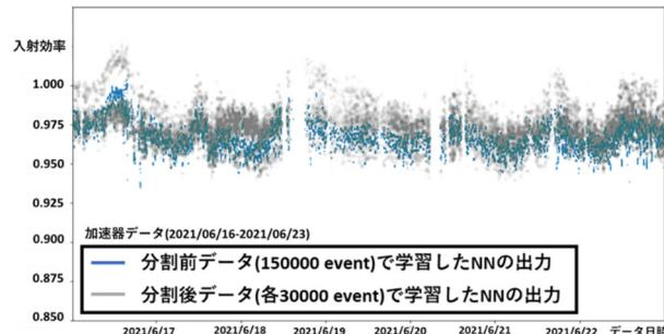
Figure 11: Predicted injection efficiencies (Q-ratios) by DNN with the whole dataset (i) (blue) and divided data sets (gray), for 2021 June evaluation data. Vertical and horizontal axis indicate the injection efficiency and date, respectively.
