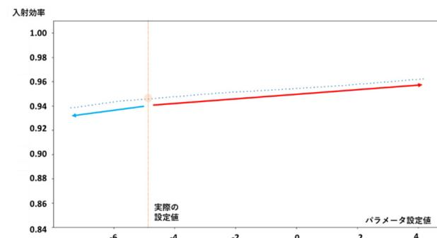
Figure 12: Predicted injection efficiency (Q-ratio) by DNN (vertical) vs accelerator parameter value (Steering magnet current for sector 3) (horizontal). The predicted injection efficiencies are obtained by DNN by varying the input Steering magnet current for sector 3.
