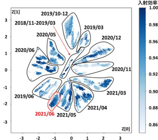
Figure 9: VAE output (two-dimensional Latent variables) from the 2018 Nov to 2021 June accelerator data. VAE is trained using 2018 Nov to 2021 May data. The output results are colored according to the injection efficiency (Q-ratio) of the input accelerator data.
