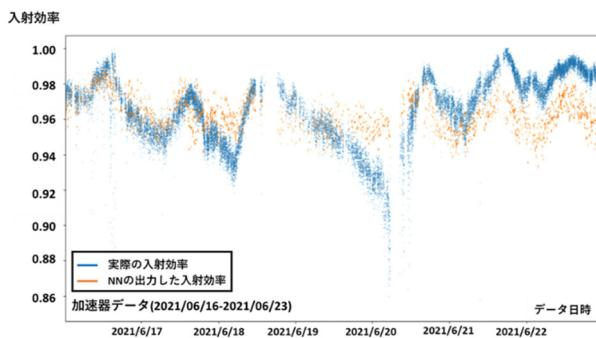
Figure 7: Injection efficiencies (Q-ratios) of predicted by DNN (orange) and actual (blue), for 2021 June evaluation data. DNN is trained using 2018 Nov-2021 May data. Vertical and horizontal axis indicate injection efficiency and date, respectively.
