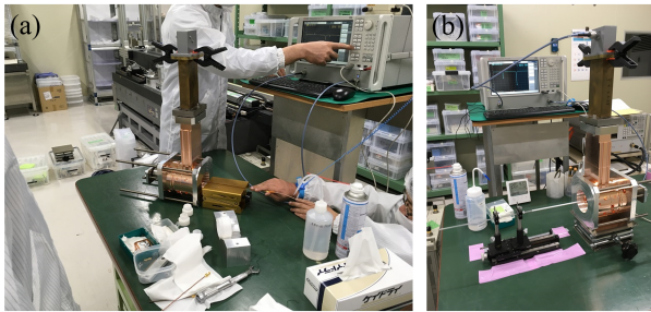
Figure 5: Photographs of (a) Resonance frequency measurement and (b) field distribution measurement.
