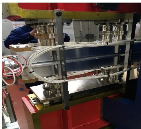
Figure 2: Photograph of the correction coil.
