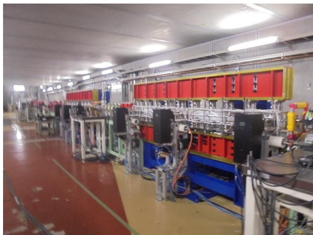
Figure 1: Photograph of the undulator U01 & U02.
