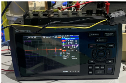
Figure 6: Data logger GL900-8 with 8Ch inputs. GL900-4 with 4Ch inputs also used.
