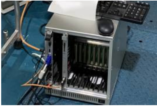
Figure 5: MTC with newly installed VME CPU.
