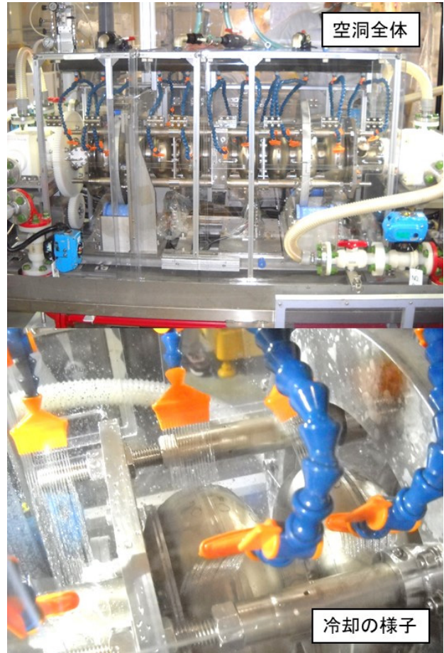
Figure 6: Upper: EP bed with water cooling system. Lower: Cooling water shower to a 9cell cavity.
