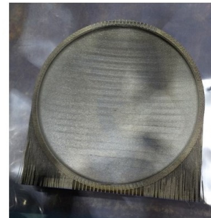
Figure 4: Pictures of the sphere window with a diameter of 60 mm and with a thickness of 0.2 mm (UP) and the window with a diameter of 166 mm and with a thickness of 0.6 mm (DOWN).
