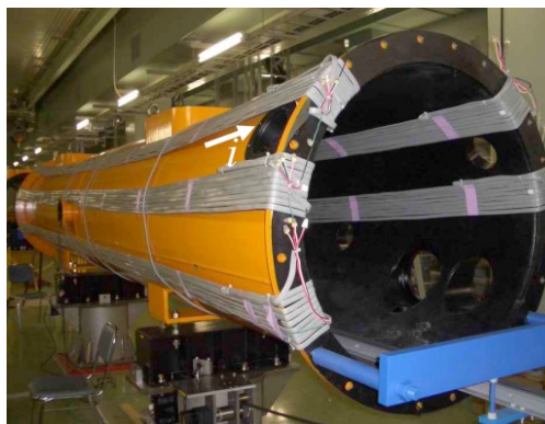
Figure 5: Demagnetization treatment setup for STF Phase I iron vessel.
