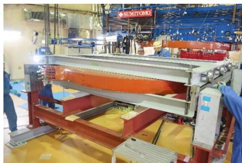
Figure 4: Removing the main coil of the cyclotron.
