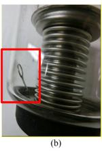
Figure 4: (a) Vacuum switch of discharge to No.2 klystron modulator (red frame: glass tube, yellow frame: solenoid coil). (b) Expanded glass tube (red frame: vapor deposition metal was whited).
