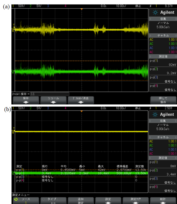
Figure 5: Output waveform of the BBA power supply with L = 0.898 mH (a) and L = 1556 mH (b). Yellow: PS Imon 1 V/A. Green: output 0.01 V/A.
