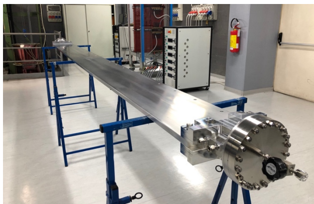
Figure 8: U#19 vacuum chamber assembly (a photo taken at SAES Getters before the NEG-film deposition).
