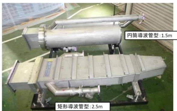
Figure 4: High power water-loads.
