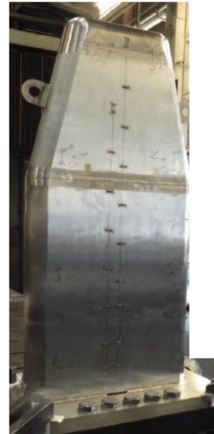
Figure 6: Hg vessel welded to the support plate. Two thermos-couples are set in the higher heating region due to spallation reaction of high energy protons and mercury on the mercury vessel.
