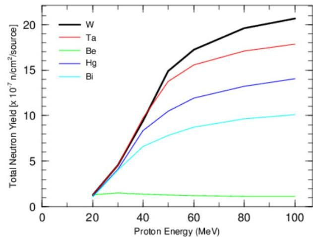
Figure 1: Total neutron yield for different spallation targets at 1 m away from the target
