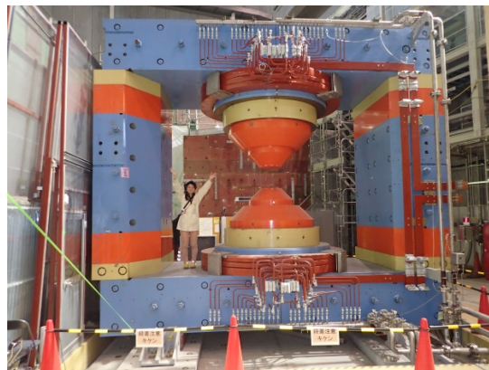
Figure 15: Installation of the FM magnet for the high-p beam line.
