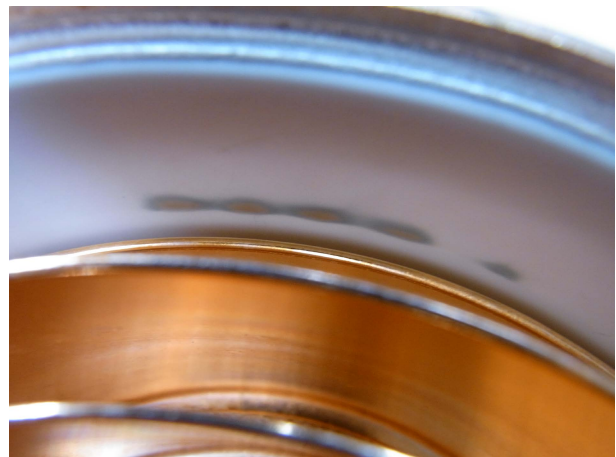
Figure 5: Discharge trace on ceramic surface.
