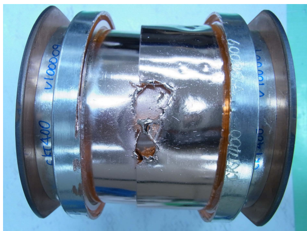
Figure 6: 400 pF vacuum capacitor (Jennings).
